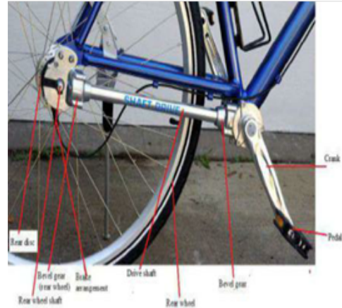
Figure 4.1 Parts of Drive Shaft
